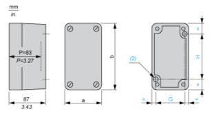
(2) 2 x Ø 5.6 mm/4.94 in. holes, depth 12 mm/0.47 in. P Usable depth
