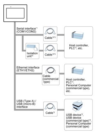
\*1 In order to use this as an isolation port, Isolation Unit is required. To use RS-232C isolation unit, set the #9 pin of the COM port to VCC.
