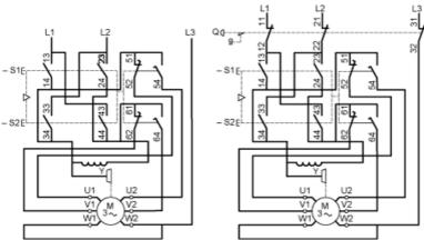
Control of Single-Speed Reversing Motor 3-Phase switching, Reversing by 2-Phase Inversion
