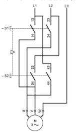
Combined with 3-pole isolating block XACS399 or XACS3991, shown in the unoperated position (pendant station "supplied"), fitted with key release trigger action latching Emergency stop operator.
