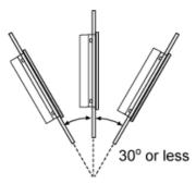
When installing the panel in a slanted position with an incline more than 30°, the ambient temperature must not exceed 40 °C (104 °F). You may need to use forced air cooling (fan,A/C) to ensure the ambient operating temperature is 40°C or less (104 °F or less).
