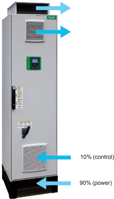
Cooling system with two separate air flows
