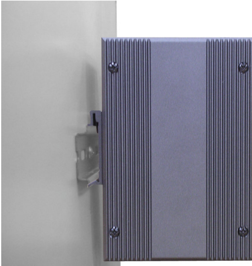
Figure 2.7: Installation to DIN-rail Step 2
