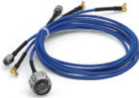
Adapter cable, pigtail 50 cm MCX (male) -> N (male), insertion attenuation 1.5 dB@2.4 GHz; impedance 50 Ω;
