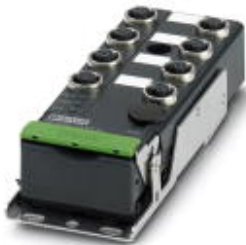
AS-i digital input/output module, AB slave, 4 digital inputs, 24 V DC, 2, 3 and 4-conductor connection method, 4 digital outputs, 24 V DC, IP67 protection
