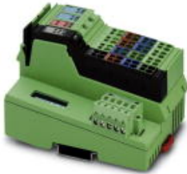
DeviceNet™ bus coupler, 8 inputs, 24 V DC, 4 outputs, 24 V DC, 500 mA, complete with I/O connectors
