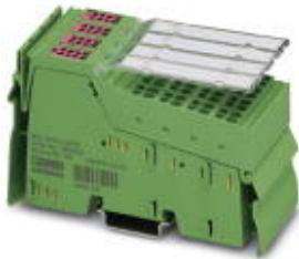
Inline digital output terminal block, complete with accessories (connector and labeling field), 32 outputs, 24 V DC, 500 mA, single-wire connection method
