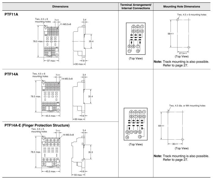
Note: If you use the PTF08A, PTF08A-E, or PT08 with an LY1 Relay, connect the following terminal pairs: 1-2, 3-4, and 5-6 (for usage at 10 A or higher).
