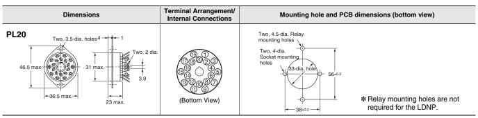
Note: When mounting, pay due attention to the direction of the key groove of applicable Relays.
