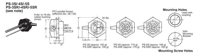
Note: The PS-3SR, PS-4SR, and PS-5SR have built-in resistor of 6.8 k $\Omega$  and used for the two-wire 61F models.
