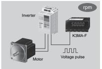
**Note:** If the monitor output from the inverter is analog, such as 0 to 10 V, use the K3MA-J.
