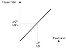
When displaying a flowrate (e.g., in #min or #h), make the scaling settings after confirming the I/O characteristics of the flowrate sensor. There are flowrate sensors that output analog signals. If this kind of flowrate sensor is used, consider using the K3MA-J.
