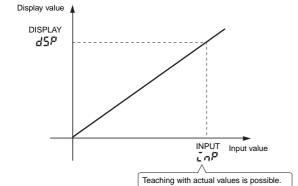
Instead of setting by inputting with the D Up Key and D Shift Key, current values can be input as scaling input values for teaching. This is useful for making settings while checking the operation status of the K3MA-F.
