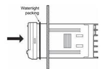
**3.** Insert the adapter into the grooves on the left and right sides of the rear case and push until it reaches the panel and is fixed in place.
