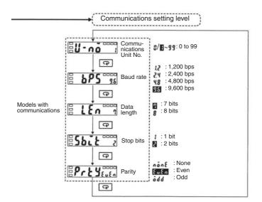
**Note:** Settings made in the communications setting level are enabled when the power is turned ON again.
