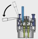
Use a gentle levering motion to lift the actuator out of the contact chamber.
