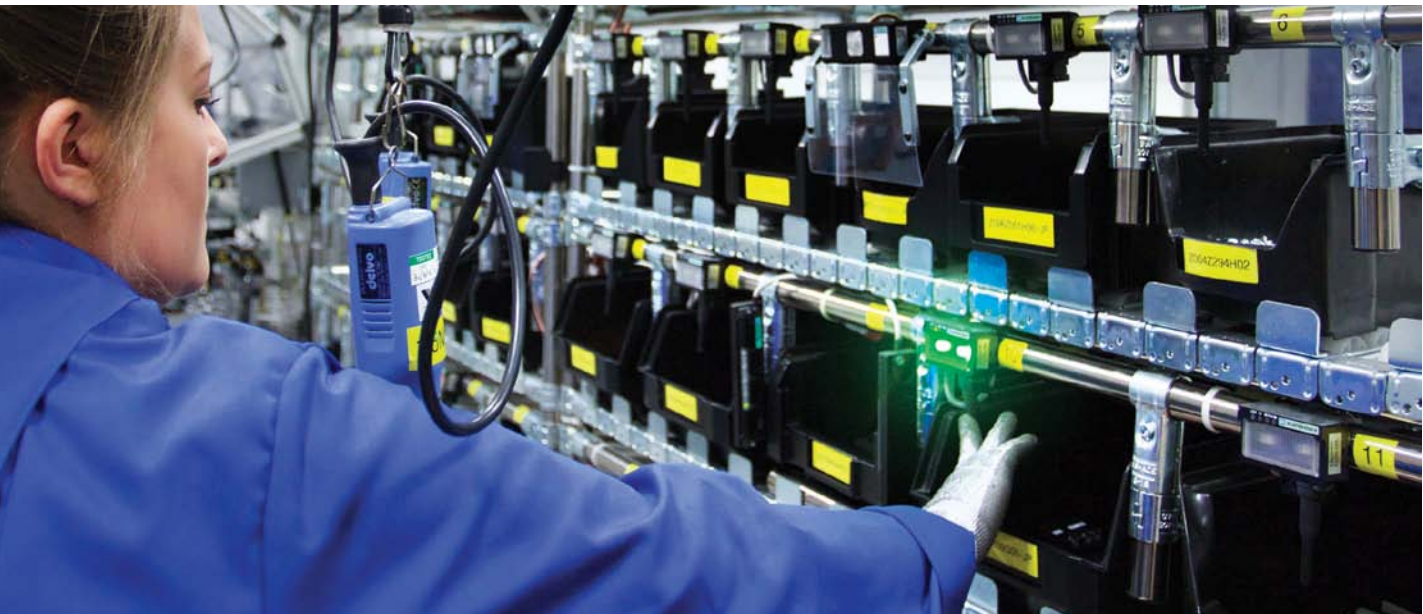
Lights or doors guide the operator to the correct box
