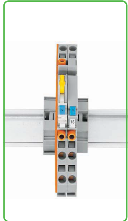
Terminal blocks required: 1 x disconnect/test terminal block 282-860 1 x through terminal block 282-866 1 x jumper, orange 282-424 1 x end plate, orange 282-386 in addition locking cover, lock-out
