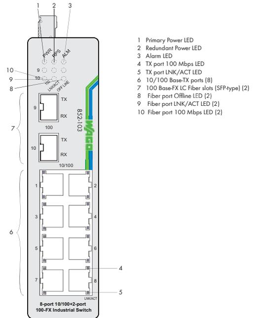
The 852-103 Industrial Switch is an 8-port 10/100Base-TX with dual SFP 100Base-FX port (SFP modules are optional) ETHERNET switch. The switch has a rugged housing, a redundant power supply and function monitoring with relay, making it ideal for a wide range of applications.
