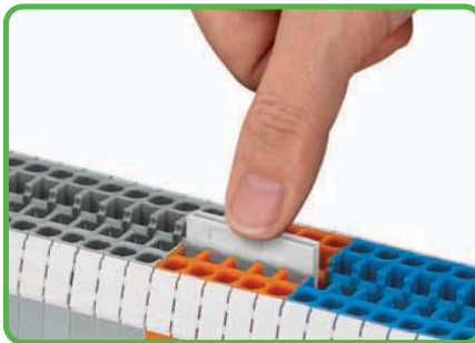
Push jumper bars down firmly until fully inserted! When using multipole bars, push alternately on right and then left side, until installed.
