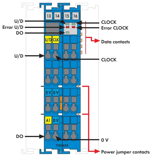
The 750-633 Counter records binary pulse signals with NAMUR-compliant levels and transmits the counter state to the fieldbus system. The U/D input allows either Up or Down counting. Counter and digital output (DO) can be set or reset via control byte. The output is short-circuit proof.
