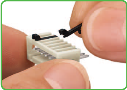
Coding a male header - fitting coding key(s).
