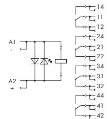
\* In order to prevent the gold layer from being damaged, these values shall not be exceeded. Higher switching power leads to evaporation of the gold layer. The resulting deposits in the enclosure may cause sparkovers between the coil and the contact.
