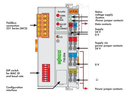
This buscoupler connects the WAGO-I/O-SYSTEM as a slave to the Device  $\mathbf{Net}^{\mathsf{TM}}$  fieldbus.
