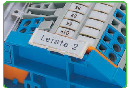
Group marking on N-busbar carrier used as end stop every 10th terminal block.
