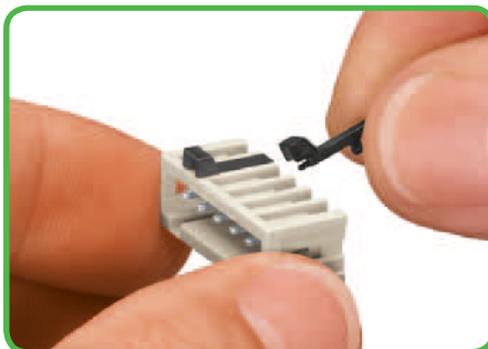
Coding a male header - fitting of coding key(s).
