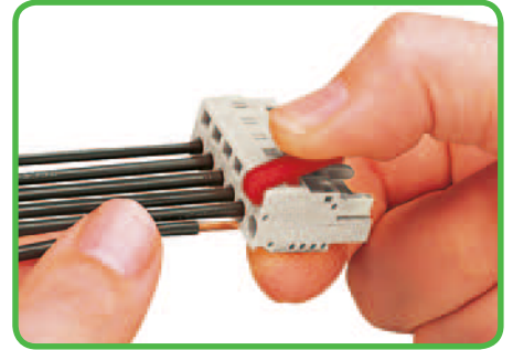
Inserting conductor - CAGE CLAMP® actuation via 231-291 push-buttons.
