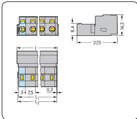
$L = (\text{pole no.} - 1) \times \text{pin spacing} + 8.2 \text{ mm}$
