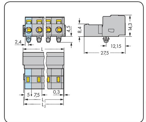
$L = (\text{pole no.} - 1) \times \text{pin spacing} + 8.2 \text{ mm}$
