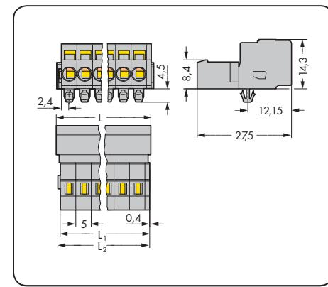
L = (pole no. – 1) x pin spacing + 8.2 mm
