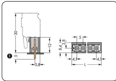
L = (pole no. - 1) x pin spacing + 8.2 mm
