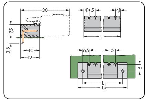
L = (pole no. - 1) x pin spacing + 8.2 mm
