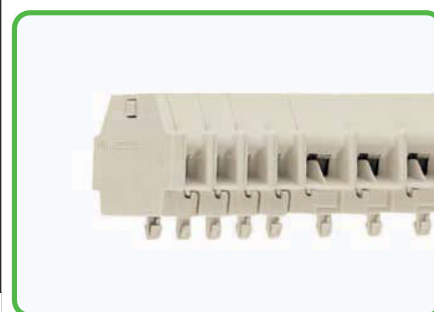
Terminal strip with snap-in mounting feet, for plate thickness 0.6 mm - 1.2 mm (0.02 in - 0.047 in), fixing hole 3.5 mm Ø (fits 210-154 aluminum rail or with 209-120 mounting adapter for DIN 35 rail)
