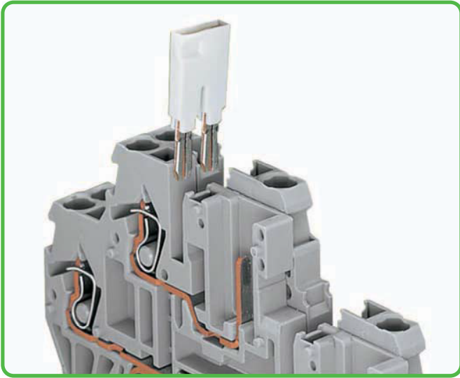
Commoning a 870-501 double-deck through terminal block with a 870-101 1-conductor/1-pin double-deck terminal block via push-in type jumper bar.
