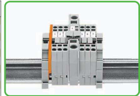
Commoning with step-down jumpers A step-down cover plate must be inserted between terminal blocks to be jumpered. Step-down jumper 284-414 commons 10/6 mm 2 /AWG 8/10 terminal blocks with 4/2.5/1.5 mm 2 /AWG 12/14/16 terminal blocks.
