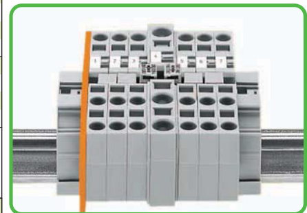
Commoning with step-down jumpers A step-down cover plate must be inserted between terminal blocks to be jumpered. Step-down jumper 284-413 commons 10/6 mm 2 /AWG 8/10 terminal blocks with 6/4 mm 2 /AWG 10/12 terminal blocks.
