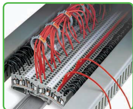
For 5 mm/0.197 in wide double-potential front-entry terminal blocks, two 3-conductor through terminal blocks are offered in one insulating housing on one level. On each side of the terminal block are marker slots for WAGO markers. Via of the available accessories, these terminal blocks can also be used as 4-conductor disconnect terminal blocks or multipliers of potential. During mounting/dis-mounting using DIN carrier rail, please note that due to the protruding webs, the terminal blocks can only be inserted or removed from the assembly after having displaced the adjacent terminal blocks (also see picture above).
