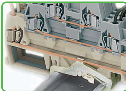
The ground conductor or shield terminal blocks have a contact foot in the bottom level, automatically establishing direct contact to the carrier rail. The flexible marker carrier, which is placed above the wiring levels, can be pushed aside during wiring or commoning. The marker carrier has three levels for three different WMB markers relating to the three decks of the terminal blocks. With a terminal block width of only 5 mm/0.197 in an effective width of only 1.67 mm/0.066 in for terminal blocks of same or different potentials can be realized for wire sizes 0.08 mm 2 - 2.5 mm 2 (AWG 28 - 14).
