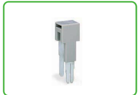
Step-down jumper commoning from 16 mm 2 (AWG 6) to 4 mm 2 (AWG 12) terminal blocks. I N 32 A 283-414
