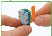
Slide locking lever into position.
