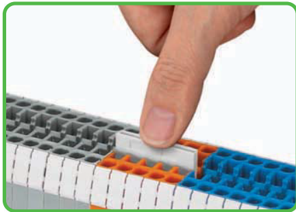
Push jumper bars down firmly until fully inserted. When using multipole bars, push alternately on right and then left side, until installed. Push-in type jumper bars 1 - 3 - 5 - 7 or 1 - - 4 - - 7 upon request.
