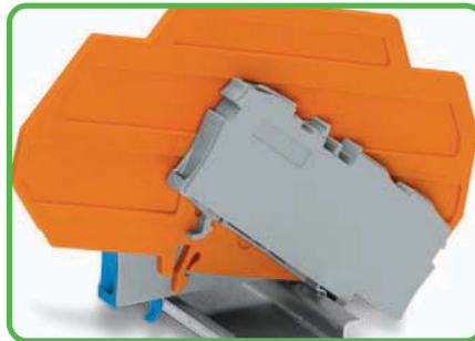
Ex e II/Ex i terminal strip Notice: The movable feet of terminal blocks and separator plate must face the same direction.
