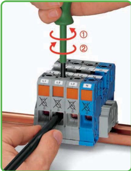
Unlock the locking tab with a short counterclockwise turn of the operating tool ①, when unlocked allow operating tool to rotate clockwise ② to securely terminate the conductor.
