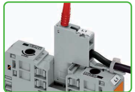
The voltage tap is inserted into the jumper contact slot. It can be fitted with a strain relief plate and provides a testing option for test plug 2 mm Ø.
