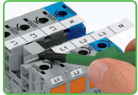
Slide the marking strip laterally to remove the jumper.
