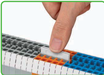
Push jumper bars down firmly until fully inserted! When using multipole bars, push alternately on right and then left side, until installed.
