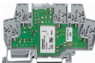
**Note:** Inductive loads have to be attenuated by an appropriate protective circuit in order to protect relay coils and contacts.
