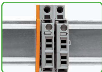
A spacer is standard equipment for 10 mm/0.394 in wide fuse terminal blocks. At the end of an assembly, or if there is no adjacent fuse terminal block, an end or intermediate plate must be used.
