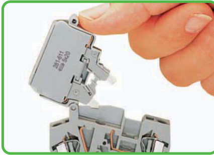
Before replacing the fuse, pivot the fuse holder in the locked open position.
