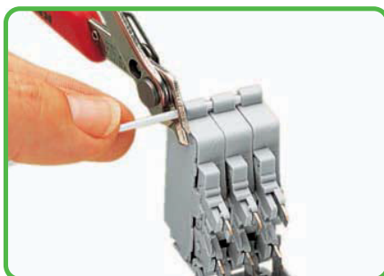
Ganging several fuse holders with a connecting strip (example: 8 mm/0.315 in terminal blocks).
