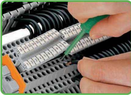
The flexible marker carrier, which is placed above the wiring level, can be pushed aside during wiring or commoning. The marker carrier has two levels for two different markers relating to double-deck terminal blocks.
