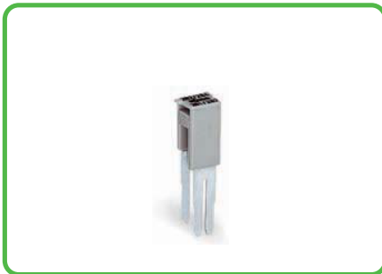
Step-down jumper commoning from 10/6 mm 2 (AWG 8/10) to 6/4 mm 2 (AWG 10/12) terminal blocks. I N 30 A 284-413
