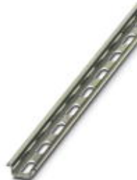
DIN rail, material: steel galvanized and passivated with a thick layer, perforated, height 5.5 mm, width 15 mm, length: 2000 mm
