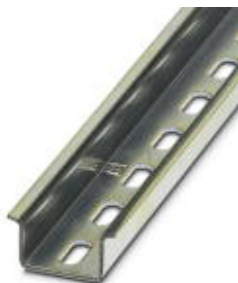
DIN rail, material: steel galvanized and passivated with a thick layer, perforated, height 15 mm, width 35 mm, length: 2000 mm
