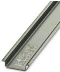
DIN rail, material: Steel, unperforated, height 7.5 mm, width 35 mm, length: 2 m
